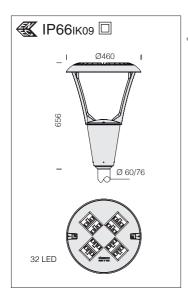
**LED:** power factor ≥0.92. Luminous flux maintenance 80%: >100.000h (L80B10).
