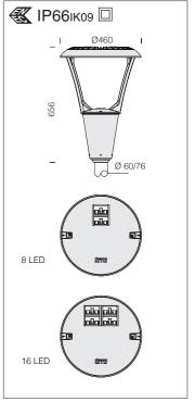
**LED:** power factor ≥0.92. Luminous flux maintenance 80%: >100.000h (L80B10).
